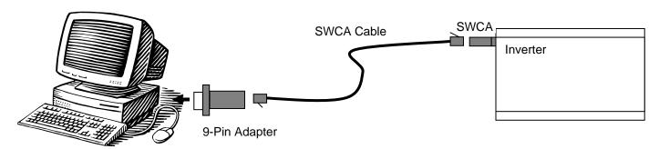
1. Begin by plugging the SWCA-II (pictured in the photograph) into the "Remote" port of the inverter. To avoid the possibility of changing the inverter's mode unintentionally as you plug it in, it is recommended to park your inverter's front panel display on the Meter's menu. The green LED on the back of the SWCA-II should illuminate when it is plugged it. It is normal for the LED to turn off by itself within 1 to 3 minutes if no PC software is communicating with the device.
