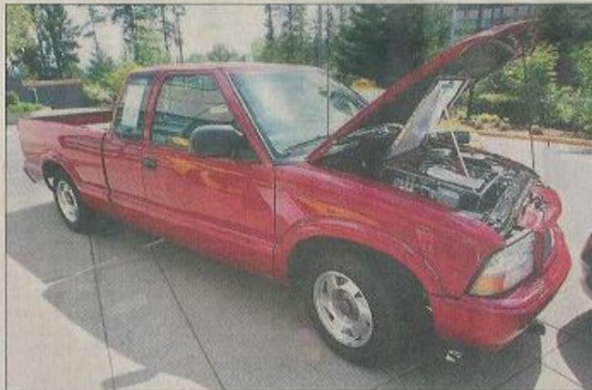
This 2001 GMC Sonoma EV Conversion truck has been converted from a gas-powered vehicle weighing 3,250 pounds to an all-electric truck weighing 4,900 pounds with a 100-horsepower electric motor and batteries.
